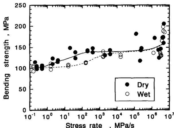
Fig. 3. Relationship between stress rate and bending strength in dry and wet conditions.
