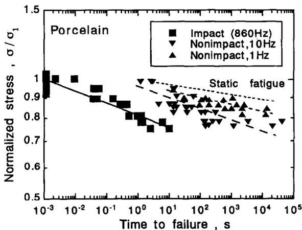
Fig. 7. Cyclic fatigue life of porcelain using normalized stress.
