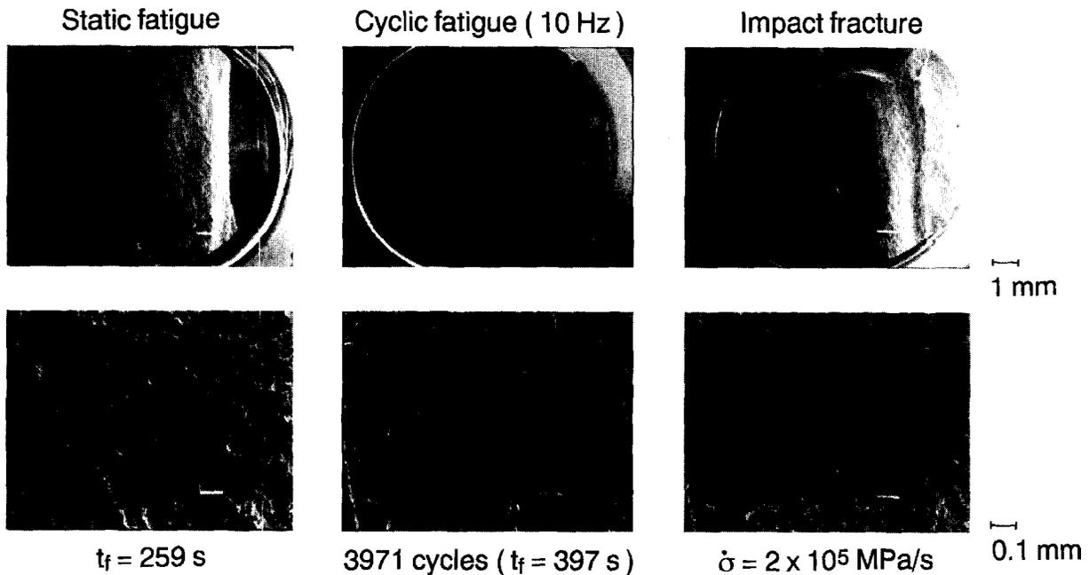
Fig. 12. SEM photographs of fracture surface in porcelain.
