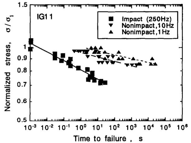
Fig. 8. Cyclic fatigue life of IG11 using normalized stress.
