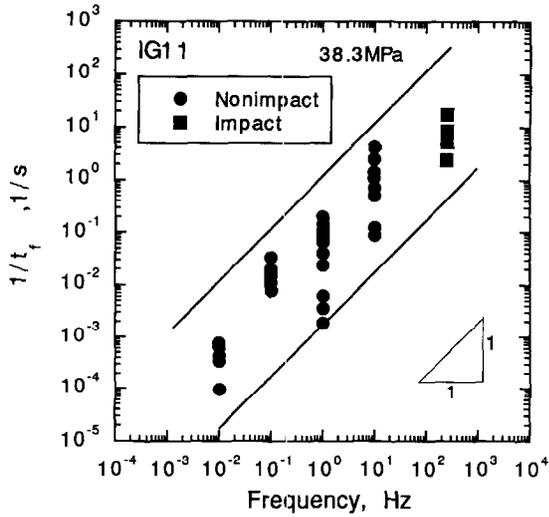
Fig. 10. Cyclic frequency effect on fatigue life of IG11.
