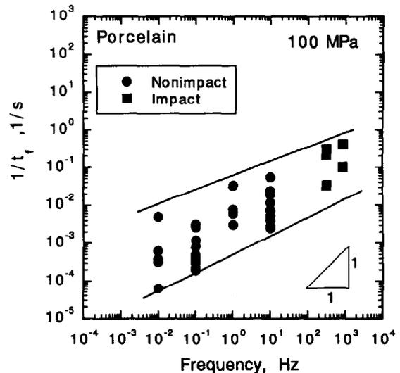
Fig. 9. Cyclic frequency effect on fatigue life of porcelain.
