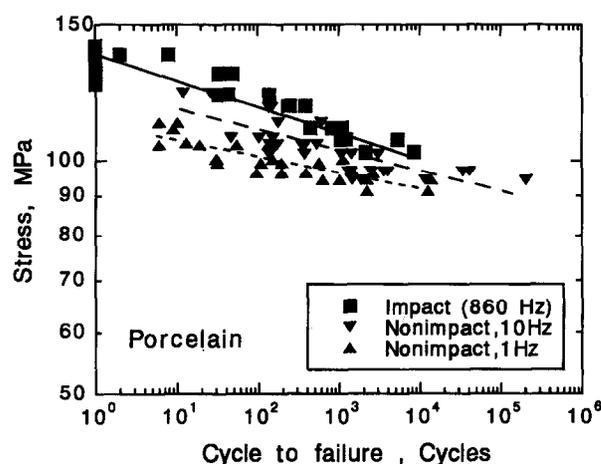
Fig. 5. Cyclic fatigue behavior of porcelain under impact load and under conventionally applied non-impact load.
